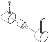
2. Use a pair of pliers to remove the cartridge by gently pulling upwards. Sometimes there is a metal ring that needs to be removed before the cartridge can be removed.
