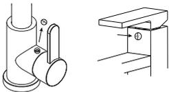
1. Find and remove the concealer cap to expose a hex screw. The concealer cap may sometimes look like a H/C cap. Then remove the hex screw to detach the handle.
