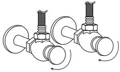
1. Turn on water supplies and check all connections for leaks. If there are leaks, turn off water supplies and check to see if proper washers were used along with proper thread sealing tape.
