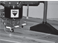
[CASTOR CHAIR TEST] ISO 4918 198 lbs. castor chair test performed to check for flooring breaks and transfers.
