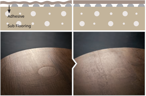
Conventional Product: Tested for glue marks and tranfer after rotating 3,000 times (Tested by LX Hausys Research Center) PRESTG: No transfers after rotating 25,000 times
