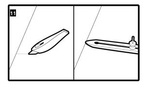
Once the cutting in the wall side is finished, place the sheet toward the wall and trim both edges.
