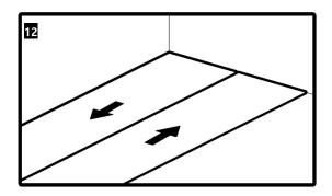
In order to match the joint areas of the sheet accurately, please use an edge trimmer. After cutting the end of the installed first sheet based on the cut second sheet, remove leftover pieces from the cut area.
