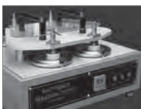
[MARTINDALE TEST] EN16094: 2012 Tested with 320 rotations on the product with a strength of 4N with a scratch pad (Scotch Brite Fleece SB7440).
